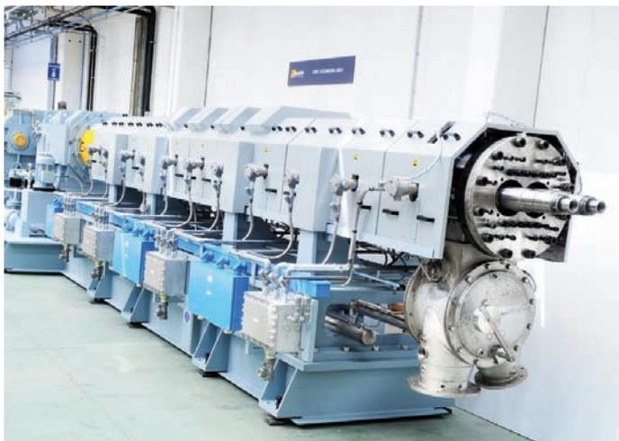
The test done at our Technological Center with the Lab. twin-screw "reactor" extruder was giving promising results. This was also possible due to our previous experiences in "reaction extruders" for other kind of process, always starting from liquid monomers for obtaining the proper reaction and a good polymer.
