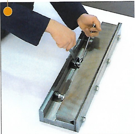
PREADJUSTMENT OF ROTATING AND FIXED BLADES
