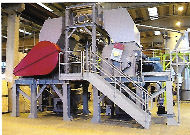
● GRINDING AREA FOR PET OR HDPE BOTTLES RECYCLING LINE COMPOSED OF TWO GRINDERS AND TWO CENTRIFUGES
